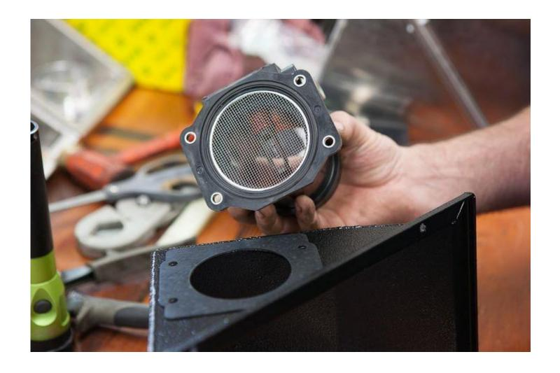
Now that you have a longer AFM mounted to the **Air Box** as opposed to the **Air Intake Adapter** you have to modify the **3" Silicone Hose 45° Elbow** that was included in this kit. You need to shorten one end of the **3" Silicone Hose 45° Elbow** by 1-1/2" total.
