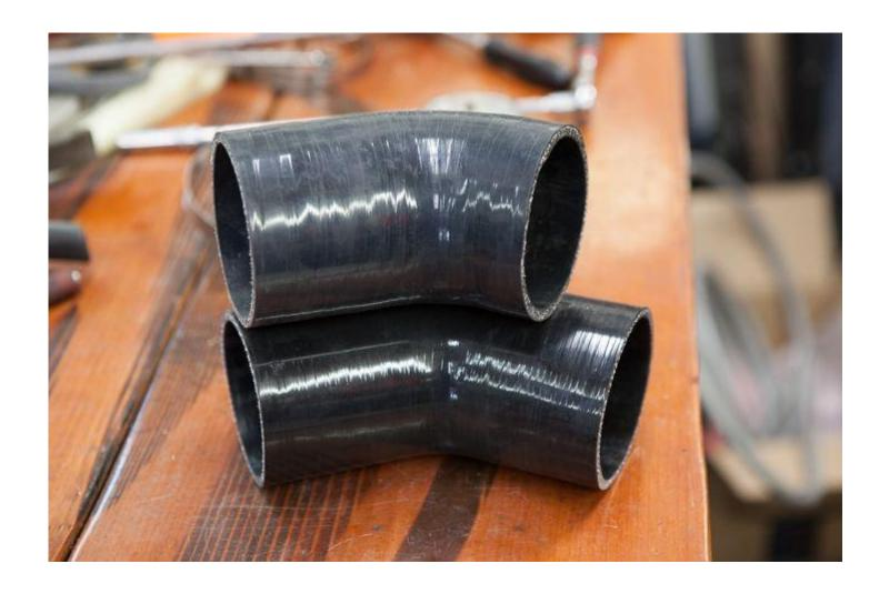
Fit the shortened end of the modified **3" Silicone Hose 45° Elbow** onto the AFM that's bolted to the **Air Box**. Fit your existing silicone elbow onto the throttle body and attach any of the remaining fittings, hoses and/or plugs to the air intake pipe.
