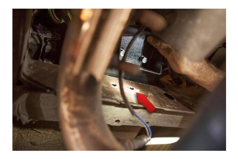
This **Backing Plate** has two hex head nuts attached to the plate in order to lock them in place while you tighten down the bolts of the support bracket.
