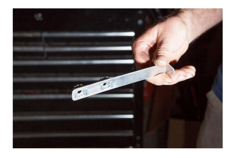
The **Backing Plate** is inserted into the larger hole next to the smaller two holes mentioned earlier. The 90° tab on the **Backing Plate** allows you to hold the plate and assist in lining up the bolts with the hex nuts.
