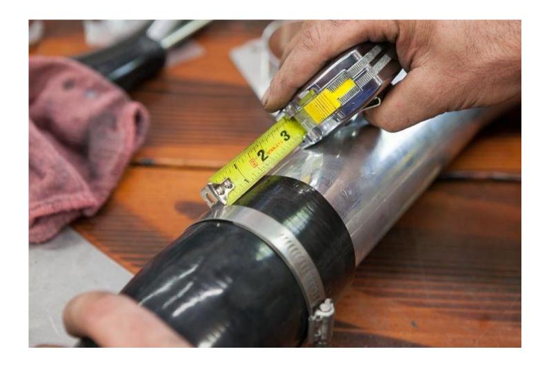
Using a **Utility Knife**, carefully cut into the **3" Silicone Hose 45° Elbow** using the **3" Hose Clamp** you've just located as a guide in order to follow around the intake pipe. This will insure that you've cut a nice square end off of the **3" Silicone Hose 45° Elbow** so that it'll mate up to your AFM perfectly.
