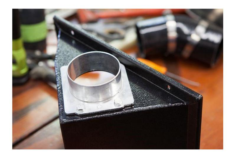
Your AFM should have a rubber seal on the base of the meter itself. Lightly grease this o-ring before bolting to the box. NOTE: the flat gasket in the photo is no longer used.
