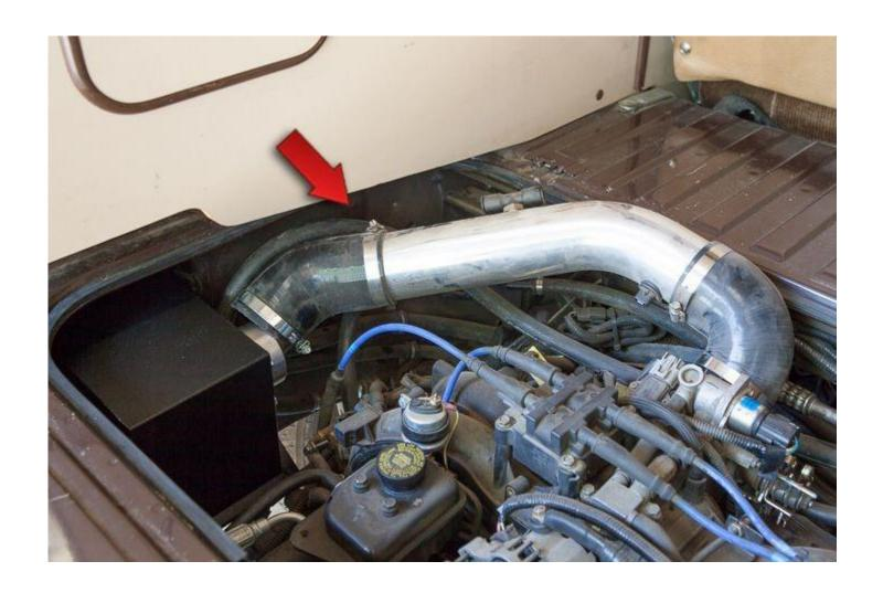
Fit the **3" Silicone Hose 45° Elbow** onto the **Air Intake Adapter** that's bolted to the **Air Box** . Fit your existing silicone elbow onto the throttle body and attach any of the remaining fittings, hoses and/or plugs to the air intake pipe.
