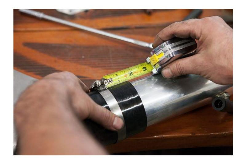
Check all around the intake pipe as well in order to make sure the **3" Hose Clamp** is exactly 1-1/2" from the end.
