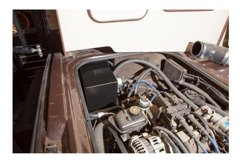
From underneath the van you'll notice there are two existing holes in the frame rail. The **Air Box** utilizes these two existing holes in order to mount to the van. If your van is older than an '85 year model you may not have these two
