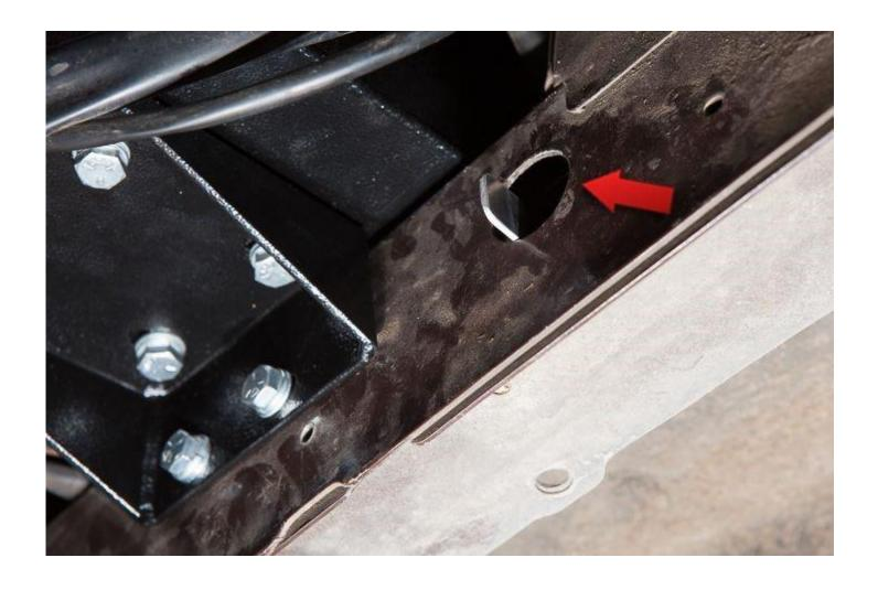
The four vertical bolts that mount the **Support Bracket** to the **Air Box** have slotted holes which will allow for some lateral, left to right adjustment. These slots come in handy in case you need to shift the **Air Box** a bit in order to work with your Subaru conversion installation.
