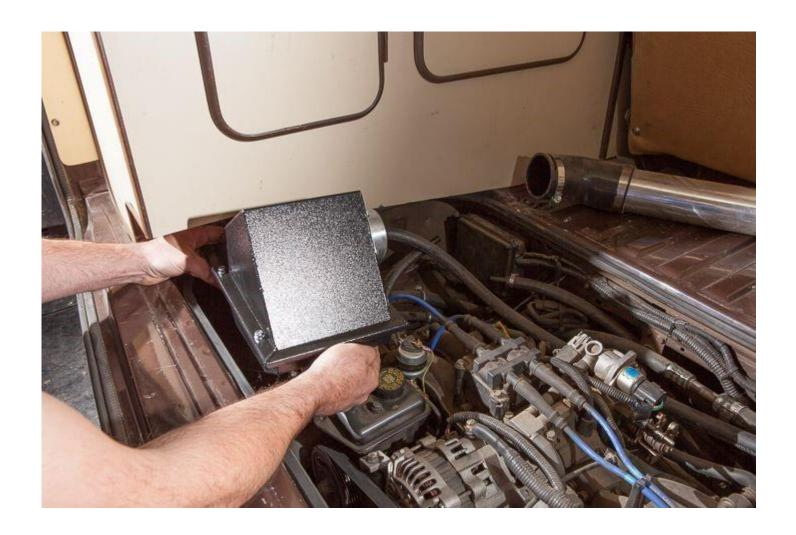
Once the  ${\bf Air\ Box}$  is in place, it should rest on the base of the engine compartment.
