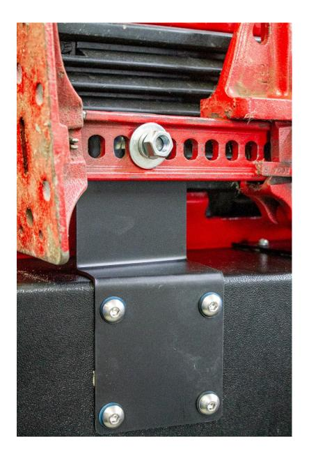
Remove the outer nut, slip on a washer, a lock washer and then reinstall the outer nut. Lift the jack slightly with your hand to center the washer in the rails of the jack and thread the nut against the lock washer. Do not fully tighten the nut. Repeat on the other side.
