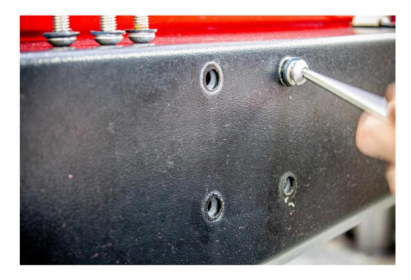
Remove the four buttonhead bolts on one side of the bumper. Clean the face of the bumper to be sure that your new Hi-lift bracket fits flat against it.
