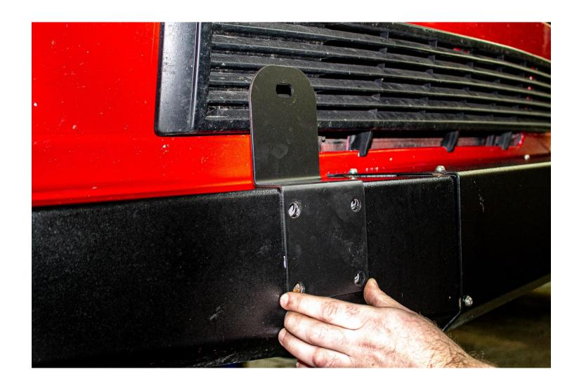
Notice that the brackets are side-specific. Choose the bracket that, when held against the face of the bumper, the upper portion is parallel to the axis of the Van. The Hi-lift jack is straight across its length and the Van has a rounded nose. Correct bracket placement will allow the Hi-lift jack to sit flush against the upper part of the bracket.
