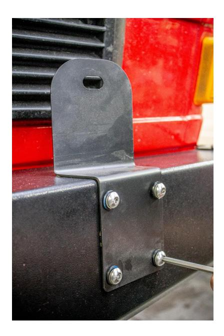
Reinstall the bolts through the bracket.
