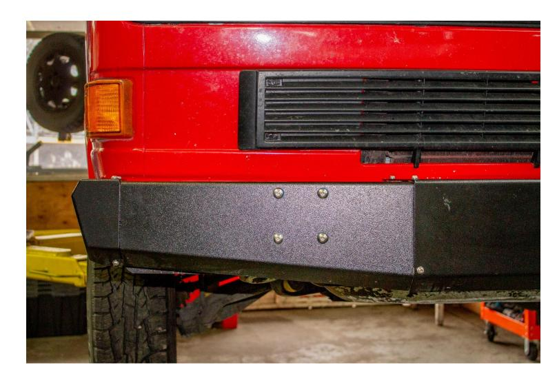
Take a moment to clean your bumper of dirt and debris. On either side of the front face of your bumper you'll find four buttonhead bolts. We'll be removing these bolts to install your hi-lift brackets. If you have Twin Peaks D-rings, these same bolts hold the D-rings to the bumper.
