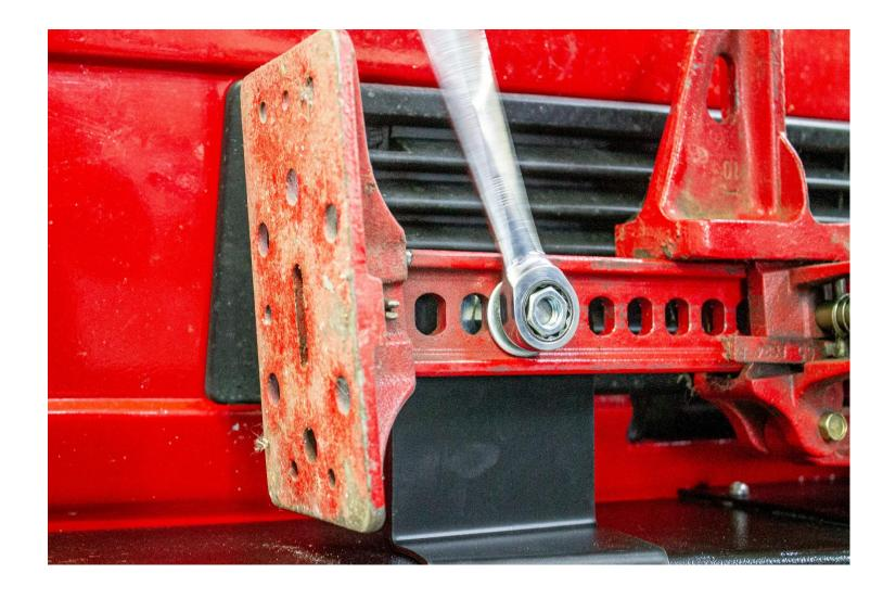
Now that the washers are centered, you're ready to do a final tightening of the outer nut. Cinch the nut until the lock washer is crushed and the nut is firmly secured. It's recommended to periodically check the torque of the nut after driving, especially after your first trip or two after installation.
