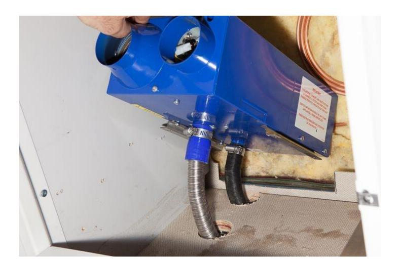
The metal exhaust line will route down through the floor and turns towards the rear of the van. It will run just alongside the stock propane tank.
