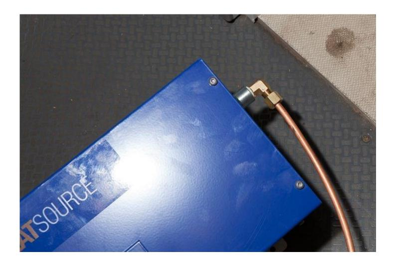
Connect the exhaust and intake lines as per the Propex instructions. Slowly feed them through the holes in the flooring. While doing this it is key to have someone under the van to help guide the lines through the floor and routed to where they need to be.
