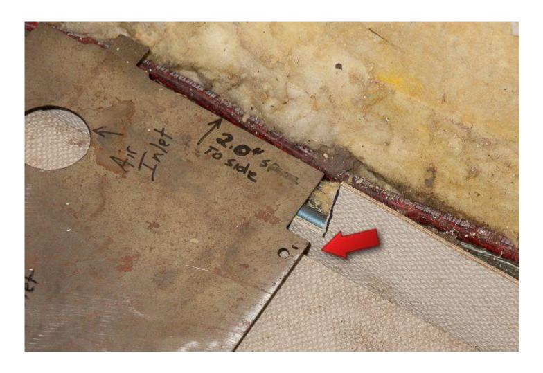
Drill the holes through the wooden floor and sheet metal floor of the van for the exhaust and intake ports per the Propex instructions. You'll need to enlarge the holes that are cut into the wooden floor of the cabinet only in order to accommodate hose clamps that secure the hoses to the bottom of the heater.
