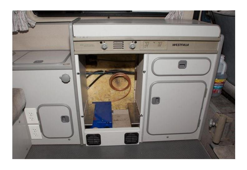
Cut a short portion of ducting and connect one end to the vent with a clamp and the other end to the Heater outlet with a clamp. These items are included in your Propex Heater Kit. The air inlet located on the right side does not need any hose routed to the other vent. Propex recommends that inlet remain open ended.
