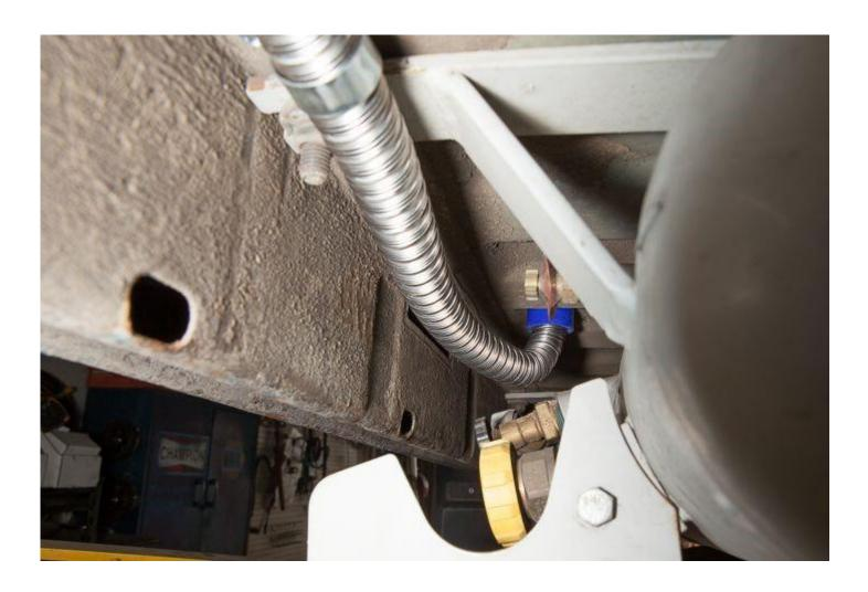
Route the exhaust line to the edge of the van. Use two Propex P-Clips in order to fasten the exhaust line to the chassis of the van.
