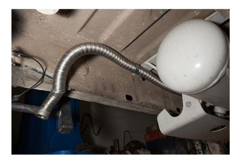
The intake line will be fed into the voided area just behind the van's side panel within the frame rail. This line needs to be routed towards the front of the van so as you feed it through the floor, have someone under the van to guide it forward. Using a **Flat Head Screwdriver** you can help route the intake line forward via the slot located in the side frame rail.
