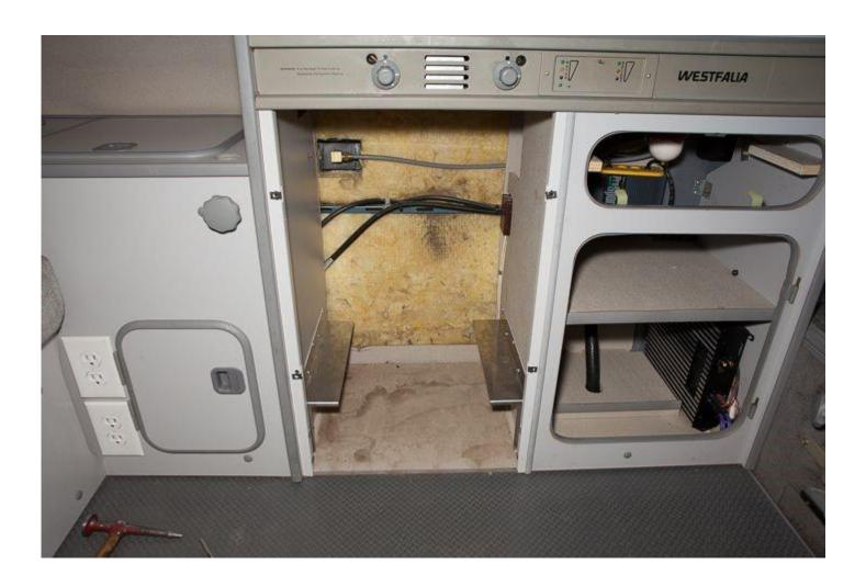
We need to remove a portion of the back fiberboard in order to make room for the Propex Heater. Use a **Measuring**Tape and a **Sharpie** to locate a vertical cut line 9" off of the left cabinet wall and roughly about 1-1/4" down from for the top edge of the fiberboard.
