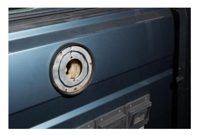
Place the **Aluminum Vent Blanking Plate** in place making sure you line up the notches in the plate with the screw holes. Reference this photo for orientation. Once in place twist the **Aluminum Vent Blanking Plate** about a half an inch and then back. This will insure that the **Aluminum Vent Blanking Plate** has a good coating of **Black RTV Silicone Sealant**.
