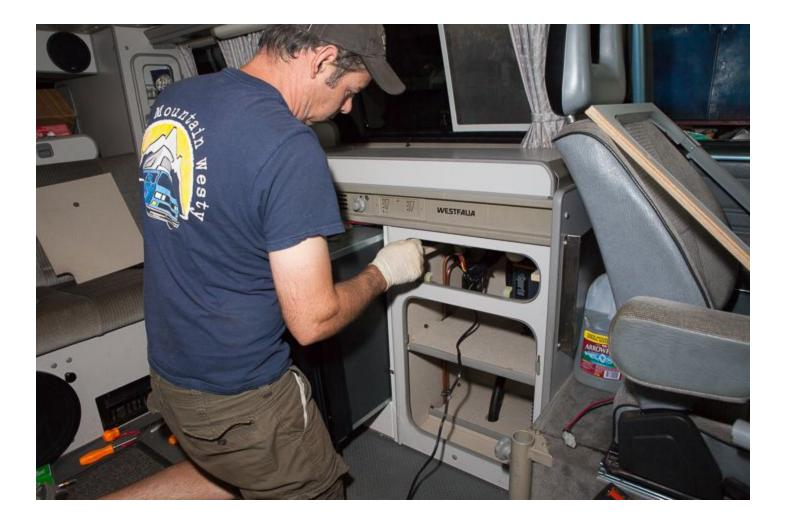
Reach through the drawer opening and into the area behind the fridge in order to grab ahold of the new AC power cord and the DC power cord that we just added the stock white plug to. Feed these through to the drawer side of the cabinet so that they're easily accessible.
