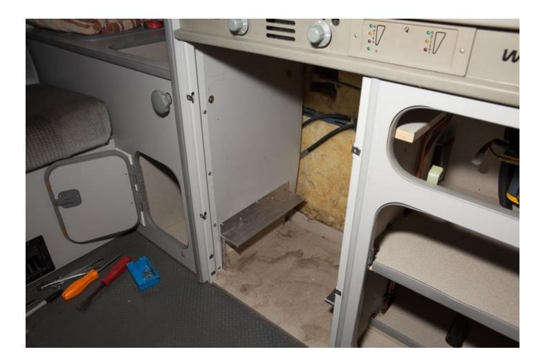
Place the **Front Face Plate** in between the two **Side Support Mounting Plates.** This fitment should be pretty snug so be careful when placing it.
