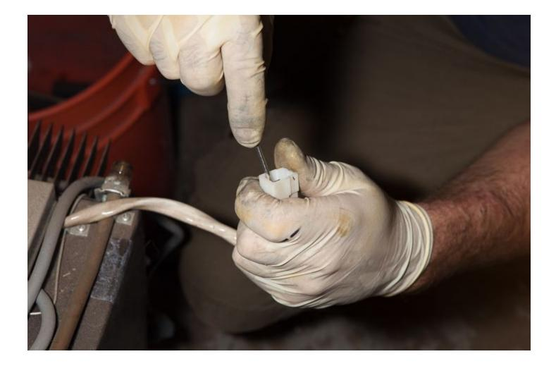
The new Truck Fridge TF49 has its own plug attached to their wiring. We need to remove their plug using a **Small Flat Head Screwdriver** to press back the small retaining clips on the wiring. Once the wires are freed we can place the Truck Fridge TF49 wires into the white stock plug that we removed from the old stock fridge.
