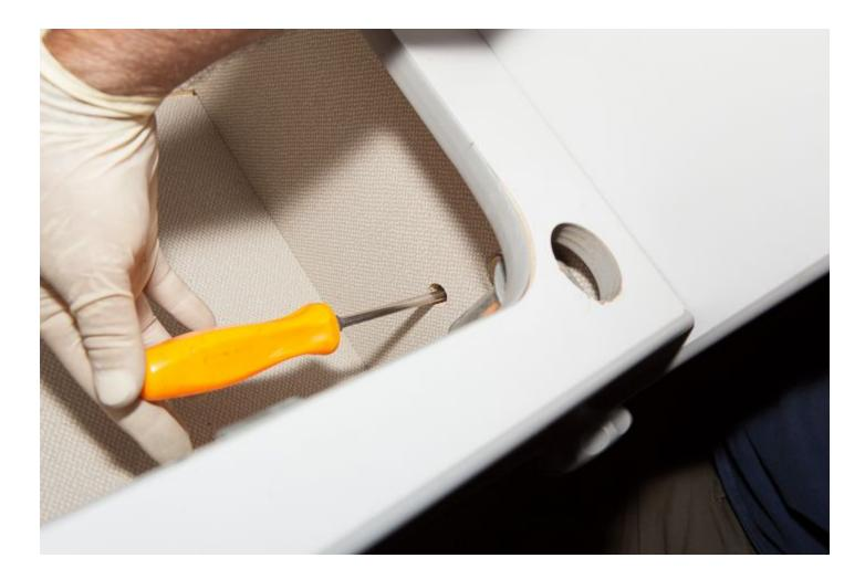
Using a **Phillips Head Screwdriver** remove the fridge mounting screw that's located in the small cubby hole cabinet area to the lower left side of the stock fridge.
