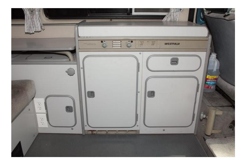
Now that the cabinet doors and drawer are removed you'll notice the AC power outlet that resides underneath the sink area. Unplug the stock fridge's AC power cord as well as the white plastic plug that supplies DC power to the fridge.
