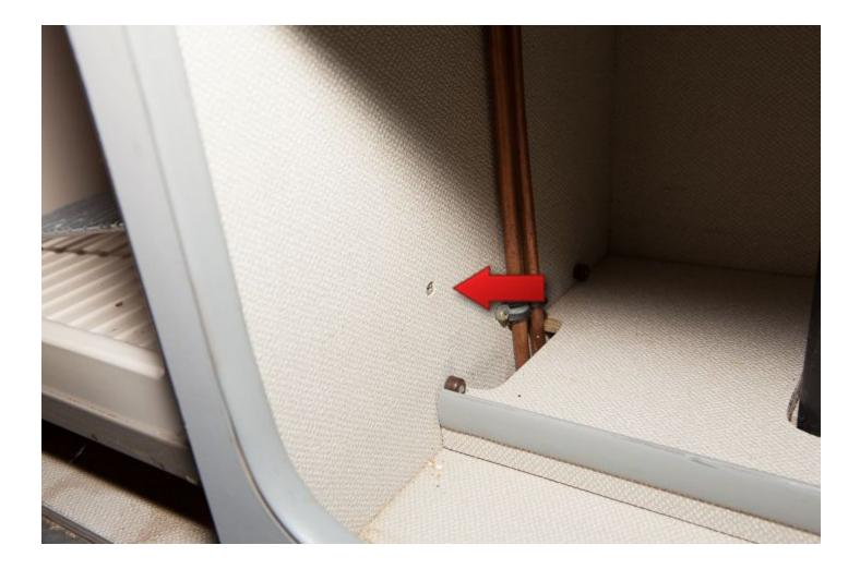
Using a **Phillips Head Screwdriver** remove the fridge mounting screw that's located in cabinet area to the upper right side of the stock fridge.
