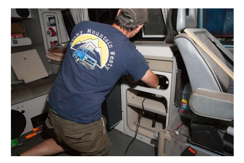
The front flange of of the Truck Fridge TF49 should fit flush against the two **Side Support Mounting Plates**. Use a **Phillips Head Screwdriver** in order to attach four **Machine Screws** from **Hardware Package C** into front flange of the fridge. These four screws will secure the Truck Fridge TF49 to the **Side Support Mounting Plates** we installed earlier.
