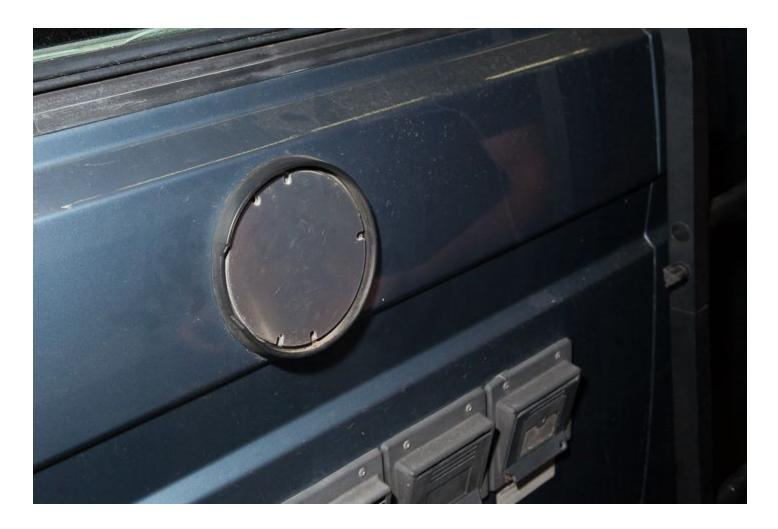
Use a **Phillips Head Screwdriver** in order to reattach the three phillips head screws that mount the Flue Vent Cover back in place.
