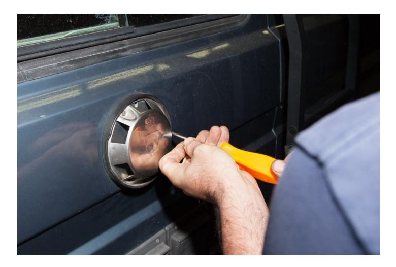
Now this Flue Vent is completely sealed since it's no longer needed for the new Truck Fridge TF49.
