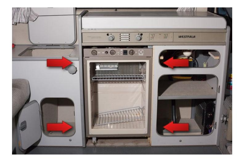
Using a **Phillips Head Screwdriver** remove the fridge mounting screw that's located in the flat cabinet area to the upper left side of the stock fridge.
