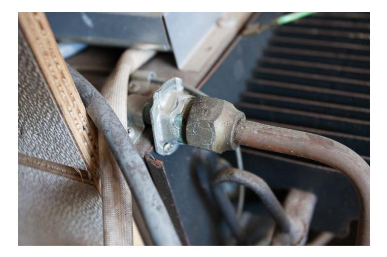
Lightly bend the disconnected propane line towards the front of the van so that you have ample access to the open end. Wrap the threads of the **Brass Plug** with **Yellow Teflon Tape** and hand thread the brass collar onto the **Brass Plug**. Use a **5/8**" **Wrench** on the Brass Plug and a **21mm Wrench** on the collar in order to fully tighten the brass collar.
