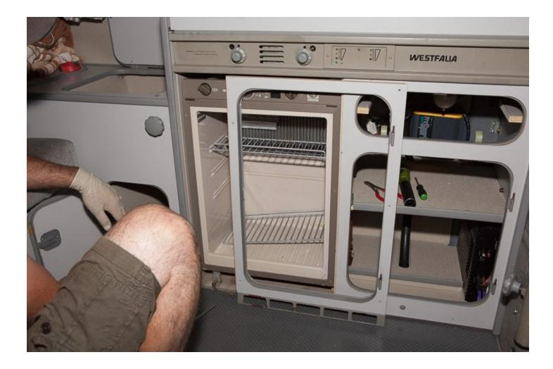
There are four screws located inside the cabinets that hold the stock fridge in place.
