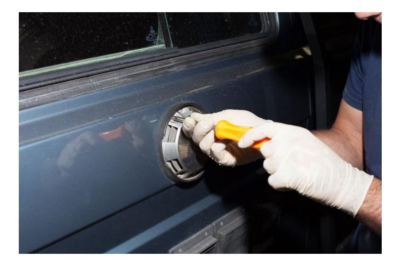
Using a **Flat Head Screwdriver** remove the two small mounting screws near the center of the Flue Vent. These screws are the last two mounting screws that hold the stock fridge in place.
