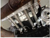
**Check clip positions:** using a ruler butted up against each downward-facing bolt, adjust the position of each clip on its tube so the two outboard clips are each 1.5" from the lower edge of the rocker chamber, and the two inboard clips are each 5" from the lower edge of the rocker chamber, as shown below left and right respectively:
