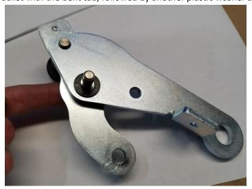
4. Next, install the small curved bracket as shown, followed by a Nylock Nut. Leave the nut loose at this time.
