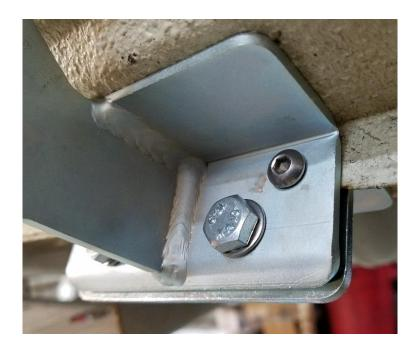
6. **(Step optional):** If you're lower pinch weld is fairly corroded, you may choose to add two #10 self tapping screws (not included) to attach the back plate to the van. This simply adds an additional attachment point for redundancy purposes.
