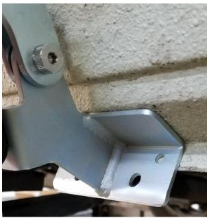
3. Attach the backing plate to the adapter using the 2 M8 x 25mm bolts, 4 washers and M8 lock nuts but leave about a  $\frac{1}{4}$ " gap. Hold the adapter tight onto the van's lower pinch weld and tighten the bolts so that the adapter is firmly held in place.
