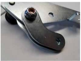
5. Install the pinch weld bracket between the other brackets making sure to put a plastic washer between each piece. Also ensure that the bracket is facing the correct direction. Add the last Nylock nut and tighten them both down. Make sure not to over tighten the nuts however. The brackets should be snug but able to move freely:
