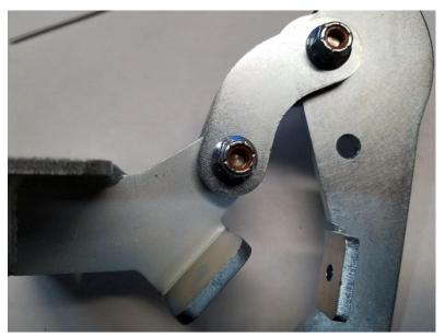
6. Next, you'll install the rubber bumper using the small #10-32 bolt and nylock nut. Run the bolt through the bumper, and attach to the bracket as shown (be careful not to over tighten!)
