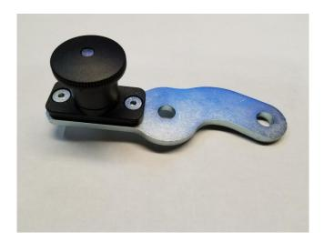
2. Next, insert one of the two shoulder bolts through the middle hole as shown, along with a plastic washer:
