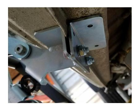
4. With the adapter securely attached to the van, you will now need to drill threw the 2 holes into the pinch weld using a ¼" drill bit. After drilling, remove any burrs and touch up the holes with some paint to prevent rust from forming.
