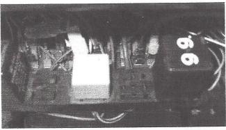
Once the fuse box has been lowered, you will be able to access the connection terminals. Be sure to complete the testing procedure on the first page to make the proper connections. Connect all wires to the "input/ supply" terminals so your headlights will be protected by the factory fuses.
