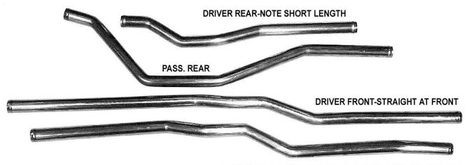
PASSENGER FRONT-NOTE BEND AT THE FRONT OF THE PIPE
