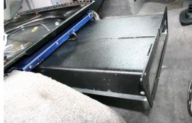
13. With the drawer frame in position and aligned, drill a couple of starter holes using a 1/16" bit. The screws provided with the kit are self tapping drill points, and a starter hole may not be necessary. Please note that all holes may not be able to anchor depending on style of van
