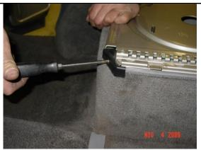
3. Gently start pulling the carpet away from the front of the seat. Take your time so the carpeting doesn't get damaged during this step. Continue to release the carpeting from the seat pedestal. Once the carpeting is loose all the way to the corner of the pedestal, tape the carpet back to keep it out of your way.
