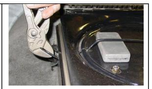
12. Remove the inner drawer from the assembly by fully extending the drawer and releasing the 2 side locks, slide the outer box assembly into the opening you just cut over the newly trimmed carpet.
