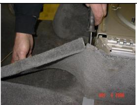
4. Carefully cut out the provided template. This will provide you with a good outline for you to follow. The template can be used for either the driver or passenger seat by flipping it over.
