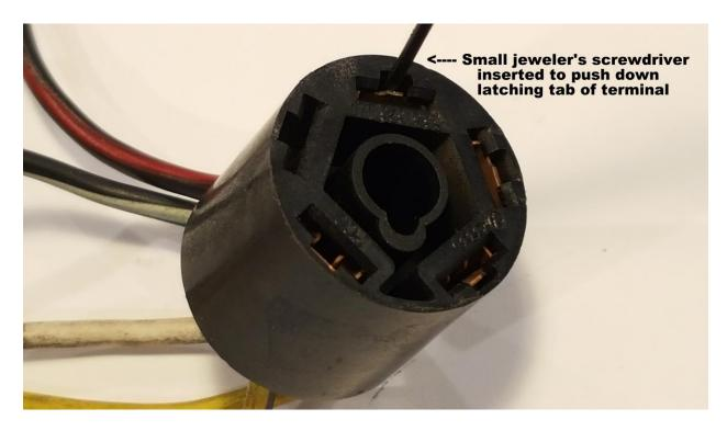
3. This shows what is going on inside the connector, where the screwdriver has pushed down the latch.
