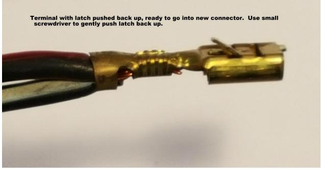
5. Reinsert terminal with power wire into fan switch connector. It should stay latched once you have pushed it in.
