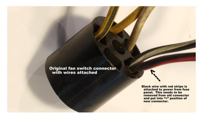
2. Insert small screwdriver into notch in connector. There are special tools available for this that work better, but they can cost \$50 or more, so we are adapting a more common tool that can get the job done. Work it carefully back and forth to press the latch down. Once the latch is depressed, the connector should slide out with the wire easily.
